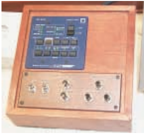
Custom control panel providing complete control over all courtroom audio
